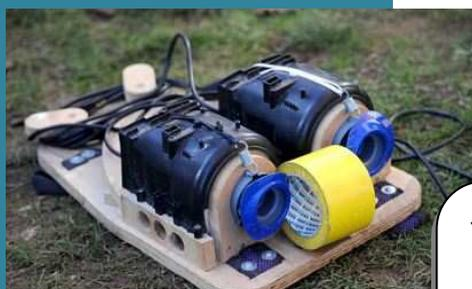
The two 1500W pumps used to suck air out of the vacuum gloves.
