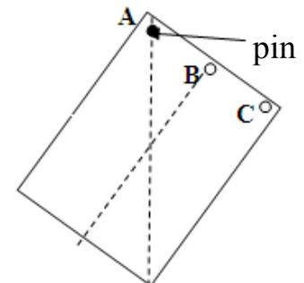
**A** A line is drawn on the card marking the position of the string.
