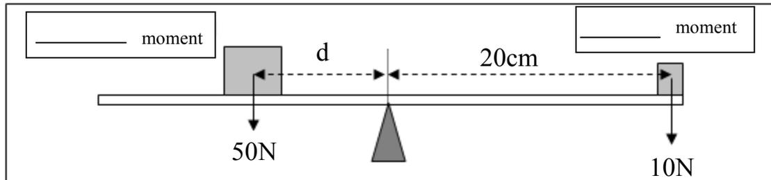
i. On the diagram above mark the **Clockwise** and **Anti-clockwise** Moments. (2)
